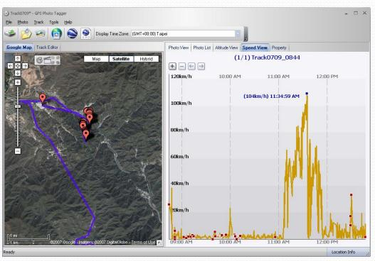
Switch to "Speed View" window will show the speed graph. The waypoints with photos on it will be marked with red square. Moving cursor on red square will display the photo.
